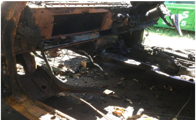
floor pan cut out after fire for car at Dalby no rust
