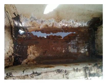
Looks like a good excuse to use the mig welder. On the other side of things, the boot floor and the right guard bottom only had a small amount of surface rust, easily sorted. The rear panel (the one that is
